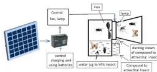
Figure 6. Diagram of trap structure
