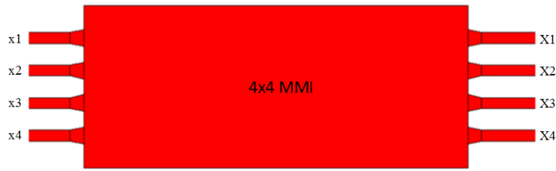
Figure 1. The structure of a 4x4 RI-MMI coupler for the KLT transform
