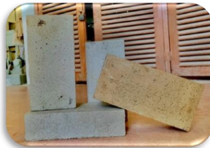
Figure 5. Brick samples are manufactured from PET plastic and glass waste
