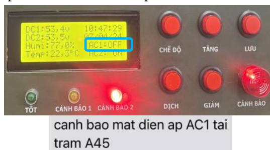
Figure 11. Respond of device when AC1 power lost
