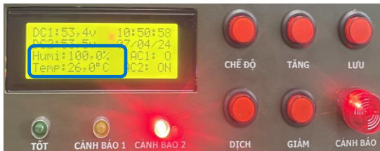
Figure 13. Respond of device when occurring temperature and humidity problem
