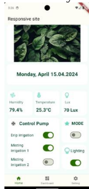
Figure 2. A screenshot of a mobile application interface designed for monitoring and controlling a growth chamber. The interface provides real-time environmental data, including humidity, temperature, and light intensity, as displayed in the dashboard.
