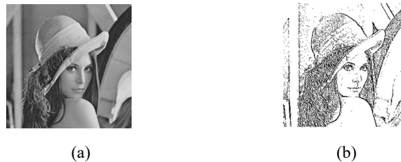
Figure 4. 256x256 'lena' images prepared for training: (a) original standard image and (b) image obtained through a 256x256 DT-CeNN using coefficients in [11]
