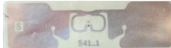
Figure 8. UHF RFID tags that can be attached to assets
