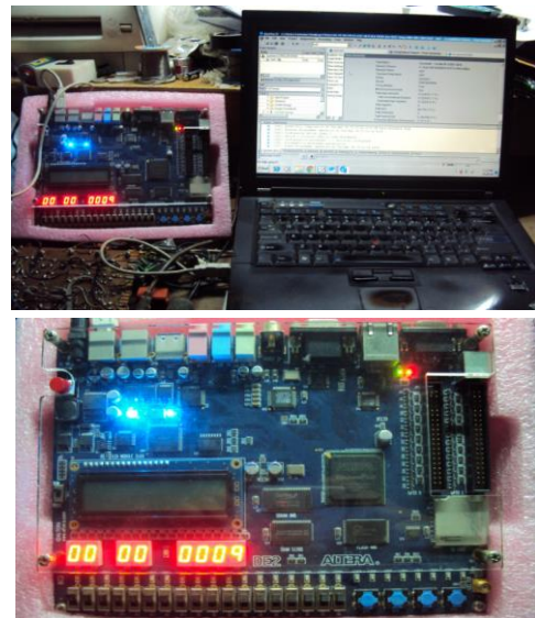
Figure 12. On the LED HEX0 of the kit DE2 shown number of objects in Figure 5 equal 9
