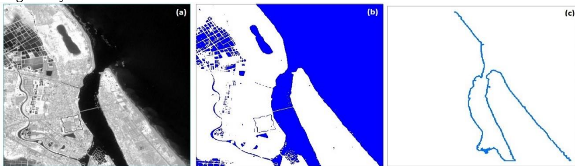
Figure 5. (a) MNDWI index image; (b) Water separation threshold; (c) Shoreline obtained
