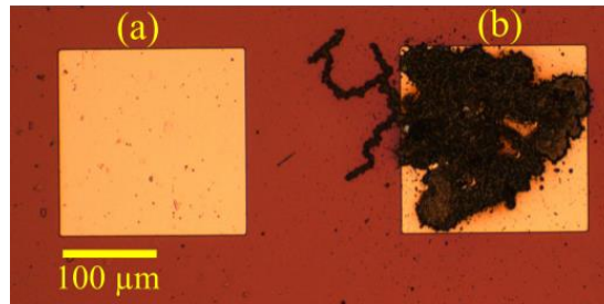
Figure 7. Optical images of PLZT thin-film capacitors with 8% La-doping (a) before and (b) after broken (under an applied electric field larger than E_{BD} value (1200 kV/cm))
