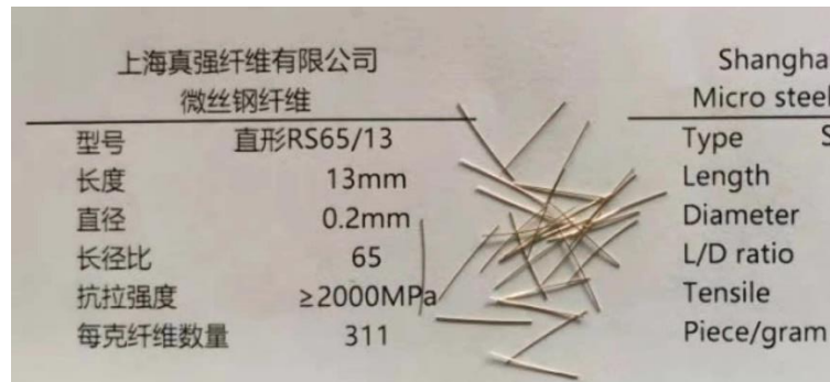
Figure 3. Steel fiber RS65/13
