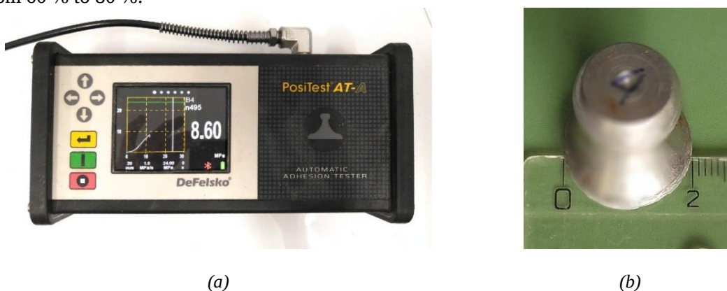
Figure 4. Pull-off device (a) and dolly (b)
