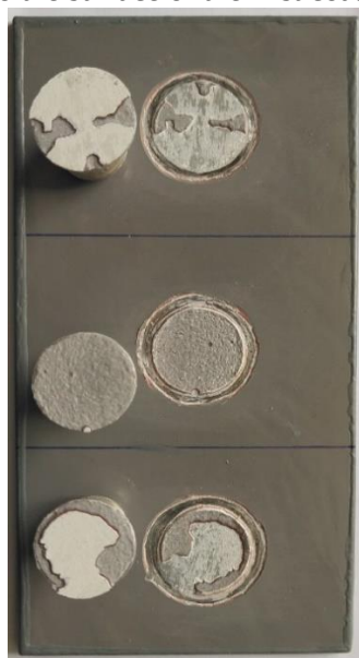
Figure 5a. Image of destruction on first coating (sample TMP2)
