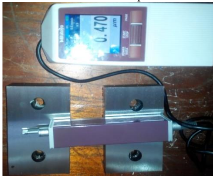
Figure 4. Image of surface roughness measurement results
