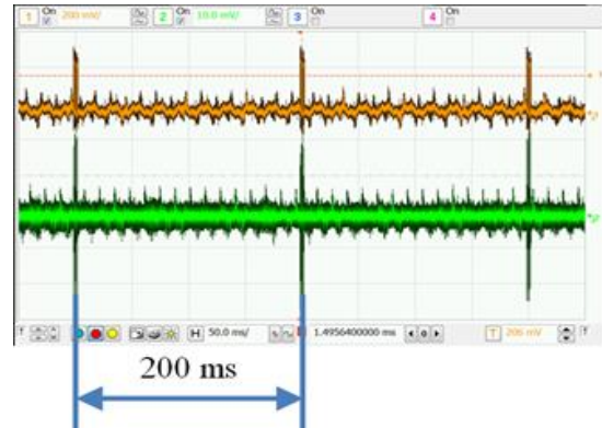
Fig. 15. Physical layer packet's frequency
