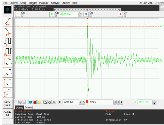
Fig. 13. Received UWB pulse
